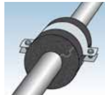
4 - Fix the collar around the support.
